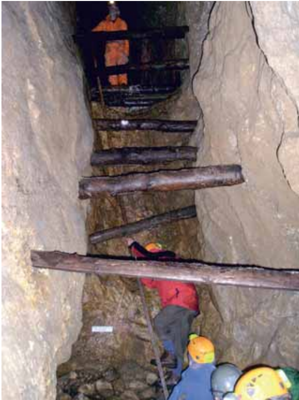
Members making their way up an iron ladder between the stemples to higher level; the footwall is on the left.
