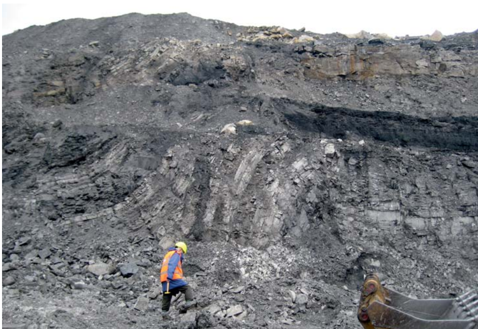
60m fault showing evidence of compression followed by extension. Tony Benfield about to add to the loose rock.
