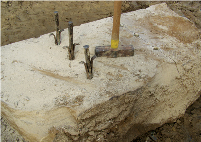
Plugs and feathers placed in boreholes ready for the quarryman's hammer to split the rock.
